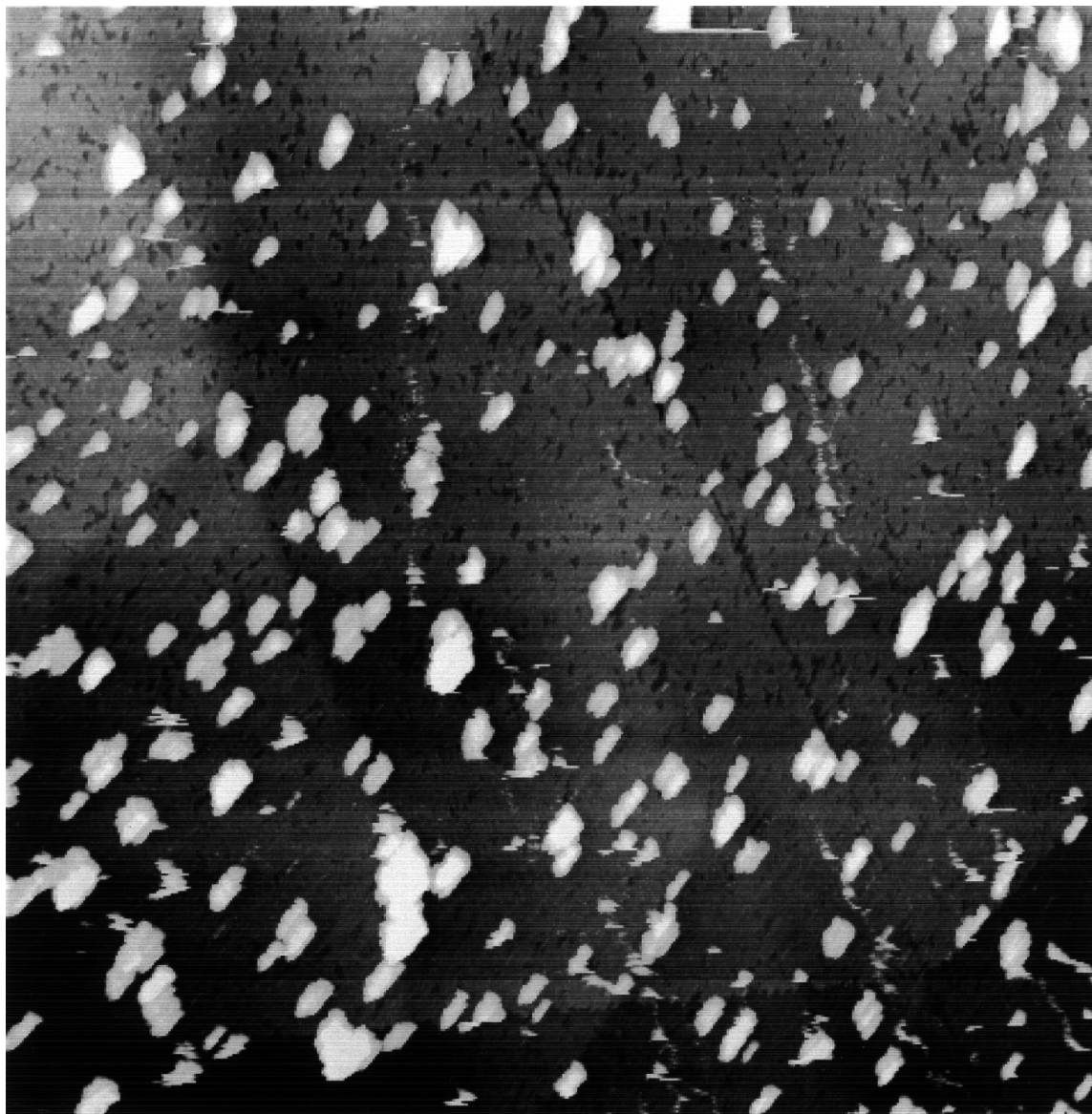
FIG. 2. STM image of the electrochemically treated sample after annealing in vacuum at 500°C for 15 min, recorded in air ( 2000 \times 2000 \text{ \AA}^2 , U_{\text{tip}} = -0.6 \text{ V} , I_t = 4 \text{ nA} ).
